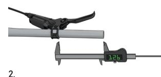
Check that there is a free and straight mounting area with a minimum length of 126 mm on the handlebar.
