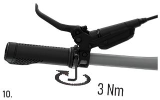
Tighten the screws with a torque of 3 Nm. The handles/grips must no longer be able to be twisted or pulled off, otherwise there is a risk of falling.
