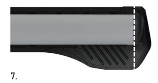
Push the handle onto the handlebar until you reach the limit stop.
